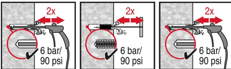
Compressed air cleaning (CAC)
